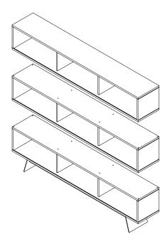
b) Place the second module on top of the first module, and align the holes. Insert an M8 conic bolt into the pre-drilled holes and into the matching metal inserts and tighten firmy with a 5mm Allen Key, but do not overtighten.
